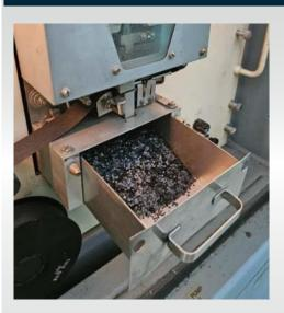
The Burroughs guidance computer on display in the LC26 Blockhouse contains several bit buckets. Look through the glass doors on the Terminal Equipment Unit and you will see little metal drawers under the recorder packages. Those are the bit buckets that collected the bits (or chads) punched out of the paper tape. In computer jargon, the bit bucket is the mysterious place on a computer where lost data goes.
