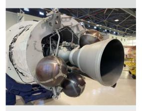
Helium – it's not just for party balloons and funny voices! Helium is the hidden hero of spaceflight. This light, non-reactive gas keeps rocket fuel tanks pressurized, engines safe, and lines clean – ensuring missions launch smoothly and crews stay protected. Without helium, history-making flights from the Cape wouldn't have left the pad. On your next visit to Hangar C, check out those spheres on the rear of the Agena A. They contained helium to support space missions.
