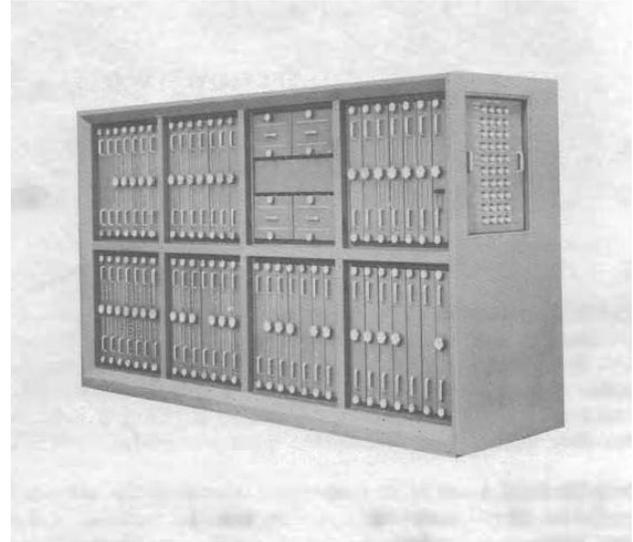
The digital computer accepts azimuth, elevation, range, range rate and lateral rate information in binary form from the rate and tracking radars. This input information is sampled by the computer and the necessary computations are performed to determine the guidance commands required by the missile on its trajectory.
