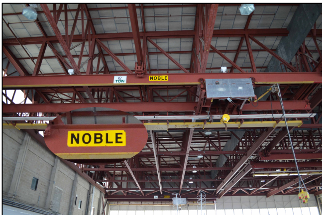
Noble (name inset) bridge crane inside Hangar R, home of the Redstone and Explorer I satellite
